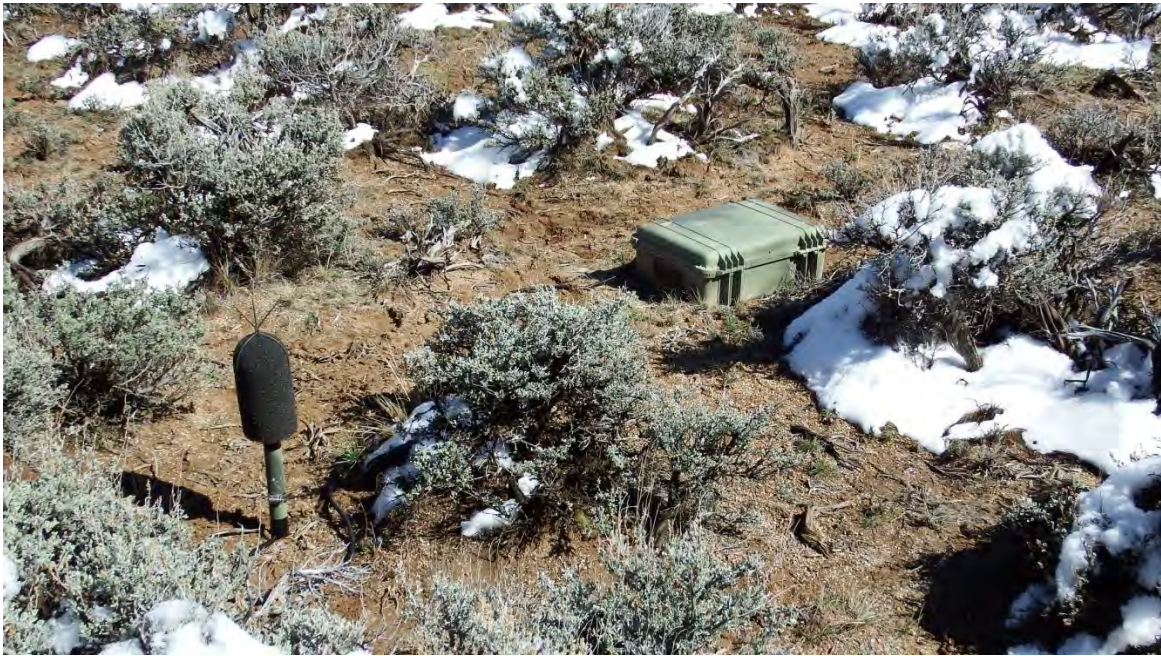
Figure 2. Typical equipment deployment near lek, showing case (sound level meter, recorder, and battery) and microphone with foam windscreen and bird spike at 0.3 m above ground.
