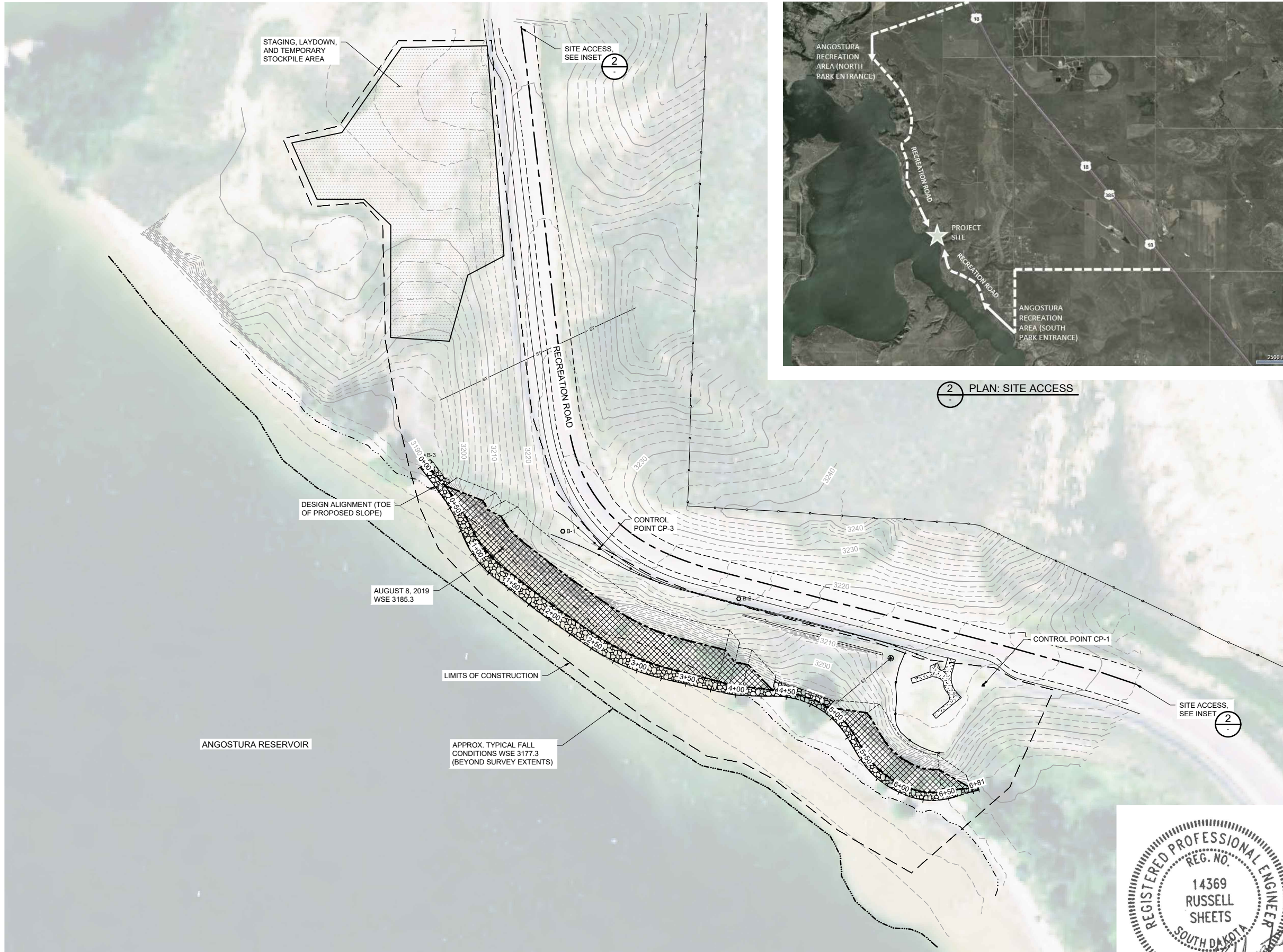
1 PLAN: STAGING AND TRAFFIC CONTROL 0 50 100 SCALE IN FEET
