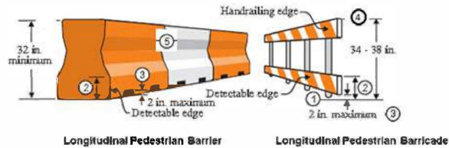
1. Barricade rail supports may not extend into the pedestrian walkway more than 4 inches from the face of the barricade.
